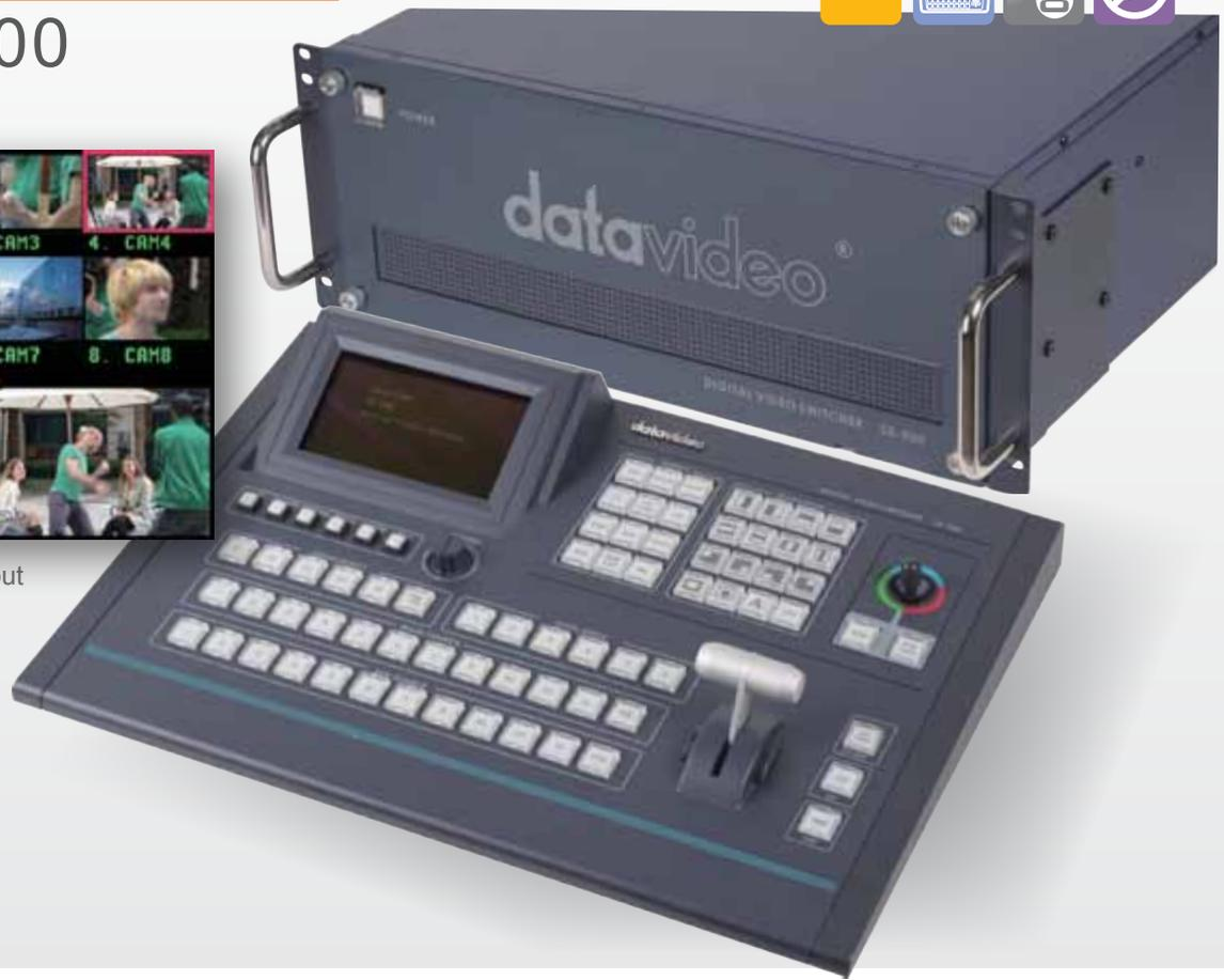
Datavideo SE-900 is a modular 8-channel SD switcher with a feature set that may be expanded with additional input cards and accessories. The two piece unit consists of a 19-inch rack mountable main frame, that holds up to 8 input cards, and a control panel. The modular switcher accepts a mix of 8 SD input of your choice including DV, SDI, DVI, YUV and Composite Video. Standard outputs
