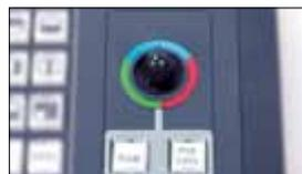
Joystick for RGB control or PiP position
