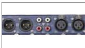
Both Phone RCA and Balanced XLR audio connection, with advanced audio delay function, assuring perfect audio and video synchronization.
